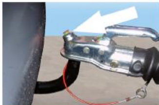
Image 5: Control indicator on the ball clutch
