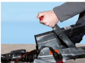
Image 7: Releasing the parking brake
