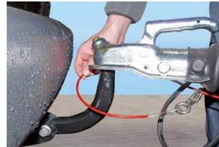
Image 6: Mounting the breakaway cable
