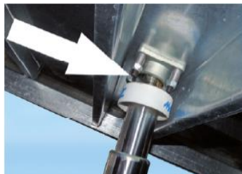
Image: Grease ball socket
