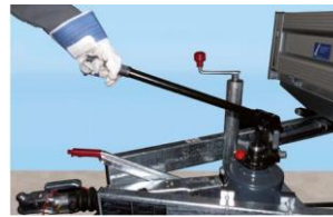
Image: Tilting the loading area
