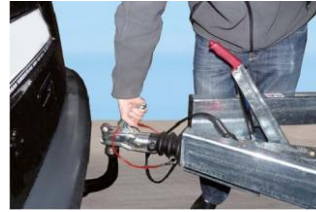
Image 2: Positioning the ball clutch
