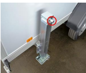
Image: Pivoting crank support
