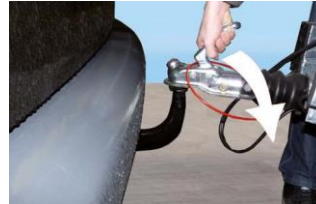
Image 4: Closing the ball clutch
