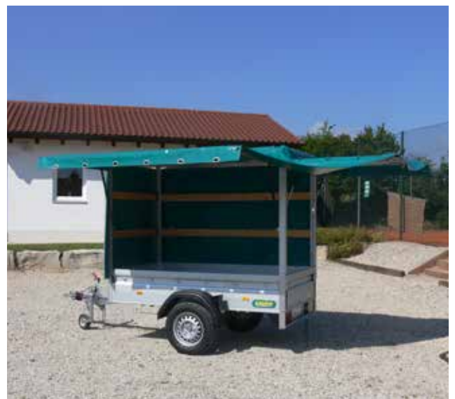
Special construction: Box trailer with tarpaulin superstructure as sales stand
