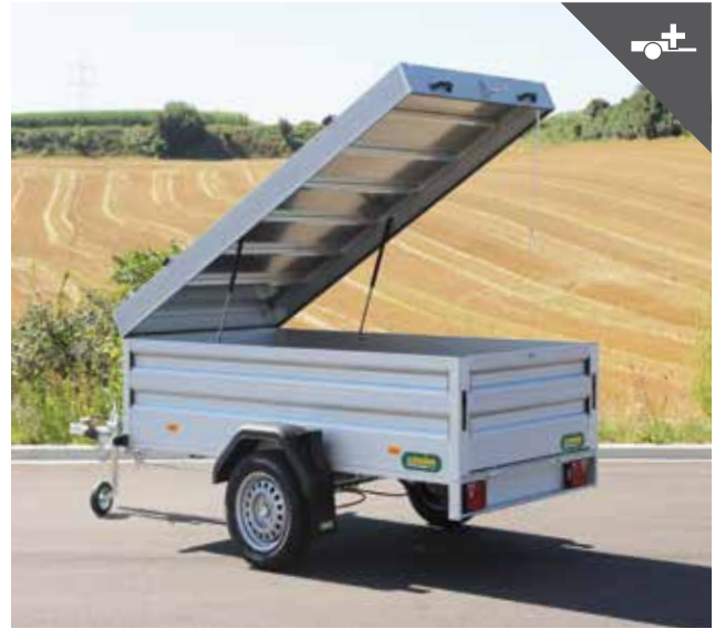
Aluminium top and side wall extension
