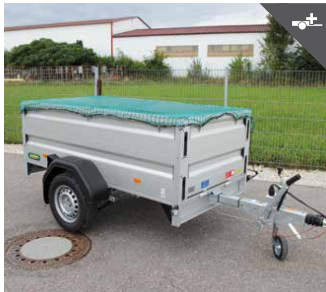
Side wall superstructure with load securing net and net hooks
