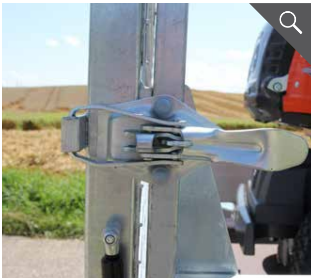
Sunken fastener for access flap
