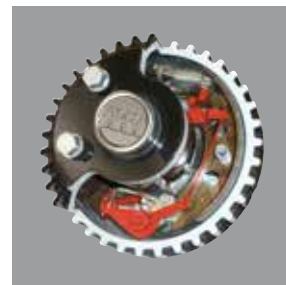
Automatically readjusting brake
