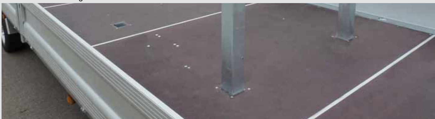
Stake pockets with plug-in stakes
