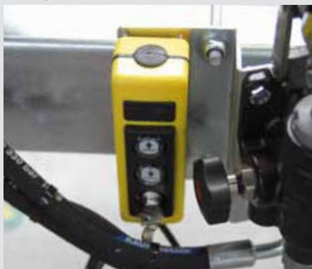
E-hydraulics operating unit can be locked
