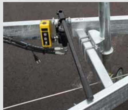
E-hydraulics with emergency manual pump
