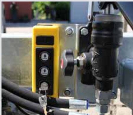
E-hydraulics with emergency manual pump
