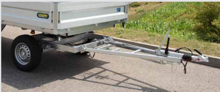
Drawbar with turntable bearing
