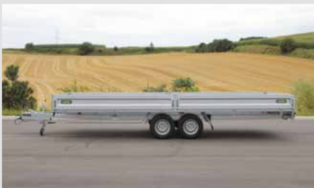
Panels with central stakes (from internal length of 5460 mm) Pluggable steel corner stakes
