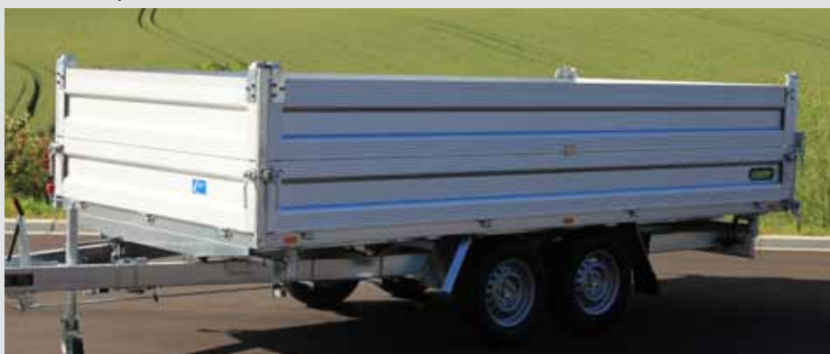
Panel extension made of the same aluminium profile as the basic panel
