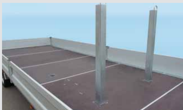
Stake pockets with plug-in stakes
