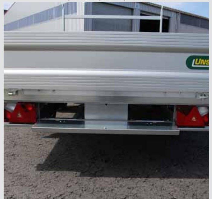
Fixture for access rails under the load floor
