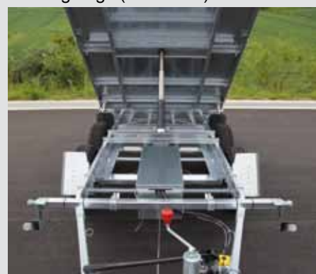
E-hydraulics installed protected
