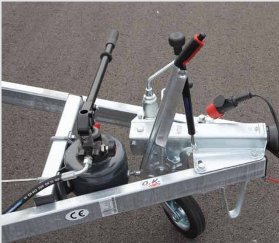
Manual pump with hydraulic tipping mechanism
