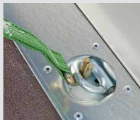
Recessed lashing point (wooden floor)
