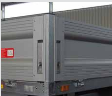
Long-lasting stainless steel fastener
