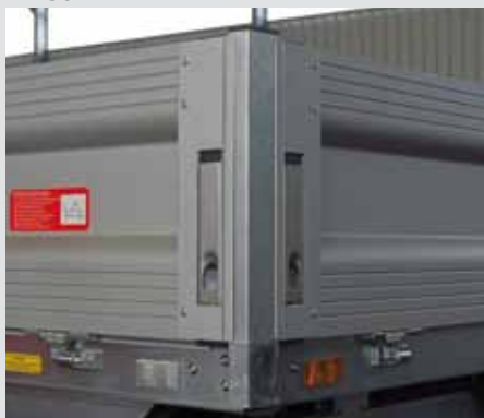
Recessed stainless steel fastener
