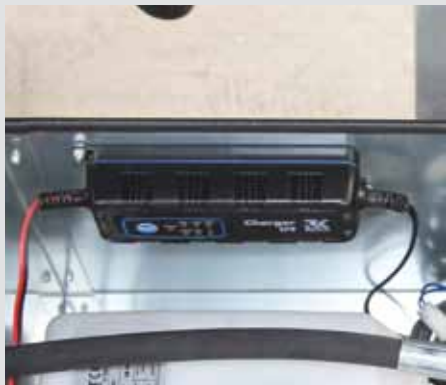
High-frequency charger with trickling charge function
