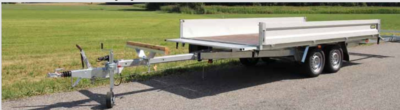
Support can be mounted in different positions on the drawbar as required
