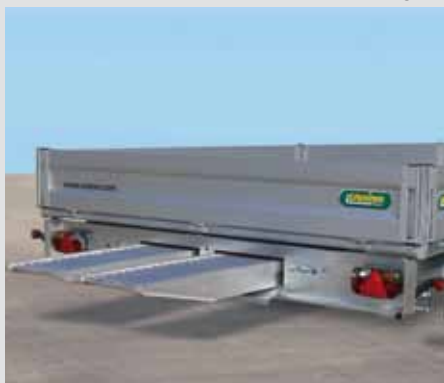
Access rails with fixture under the load floor
