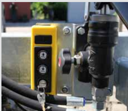
E-hydraulics with emergency manual pump
