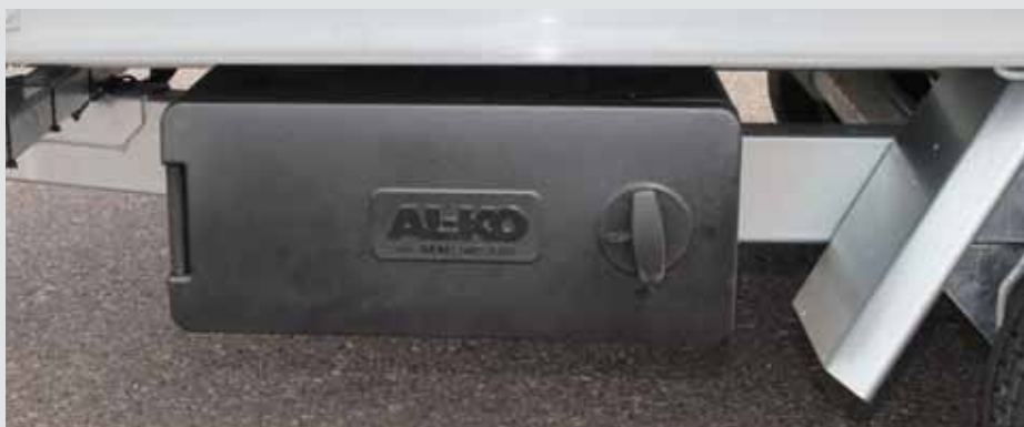
Tool box fitted under the load floor
