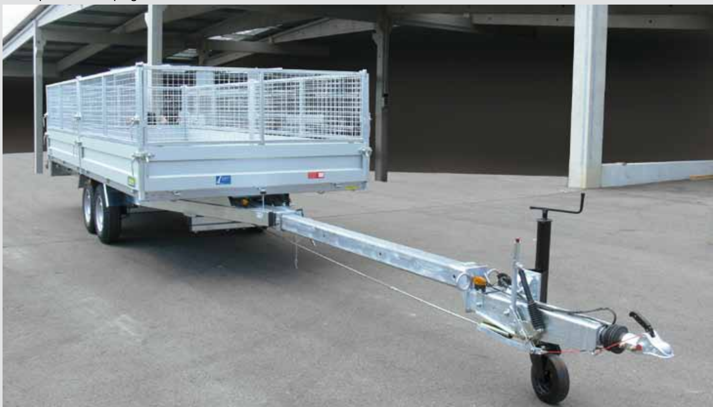
Mesh sides and drawbar in special length
