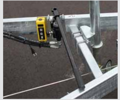
E-hydraulics with emergency manual pump
