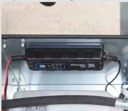
High-frequency charger with trickling charge function
