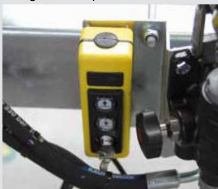
E-hydraulics operating unit can be locked
