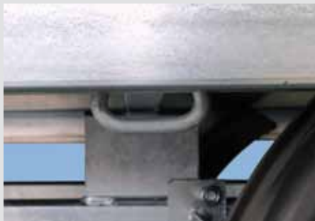
Lashing ring under the load floor
