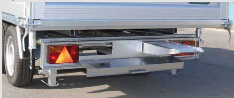
Extendable access rails with clamping fixture under the load floor
