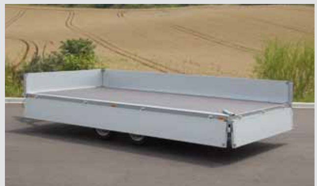
Panels with central stakes (from internal length of 5460 mm) Pluggable steel corner stakes
