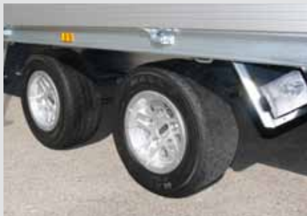
Balanced aluminium wheels
