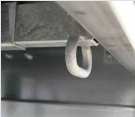
Lashing ring under the load floor
