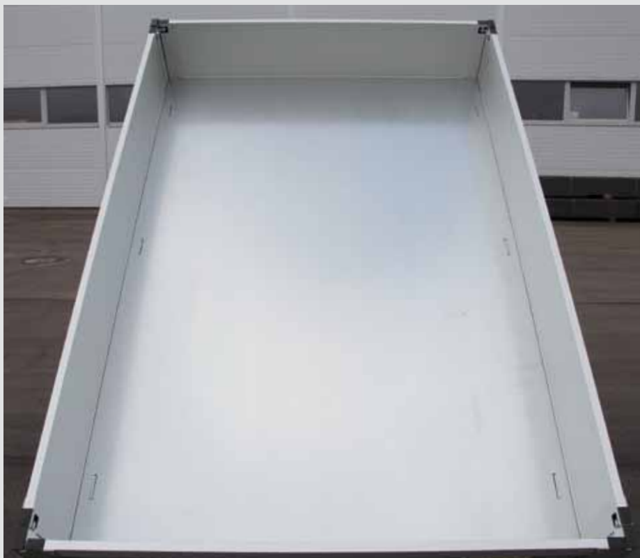
Steel floor with recessed lashing rings
