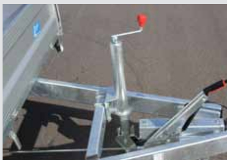
Automatic drawbar castor wheel
