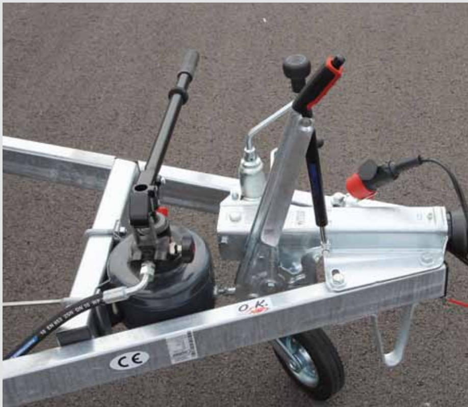
Manual pump with hydraulic tipping mechanism
