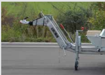
Vertically adjustable drawbar
