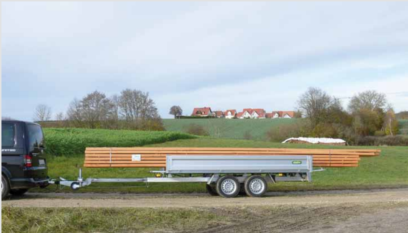
Maximum drawbar length of 3100 mm in standard version
