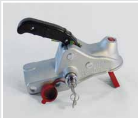
Safety ball + cylinder lock
