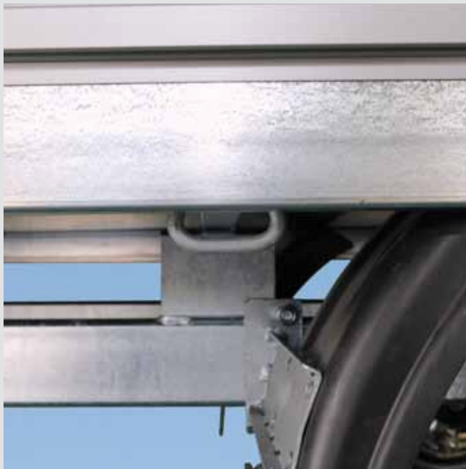
Lashing ring under the load floor
