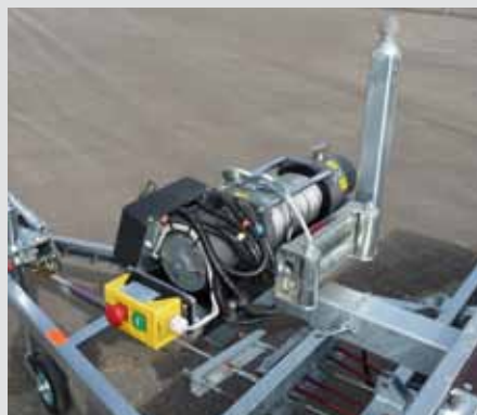
Electric cable winch
