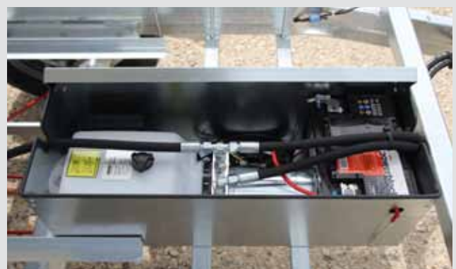
Powerful E-hydraulics with high-quality trickle charger
