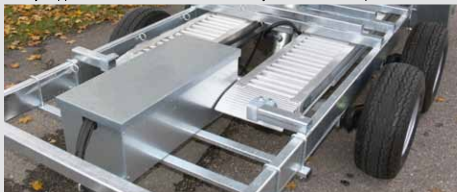
E-hydraulics and access rails
