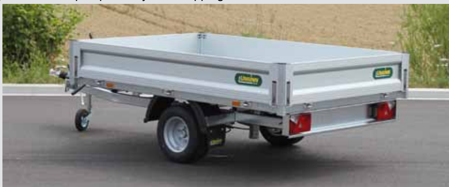
Drop-down aluminium panels
